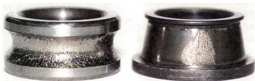
Fig. 1 Appearance of Bearing damage
