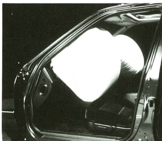
Fig. 10 HONDA SRS Airbag System when Fully Deployed
