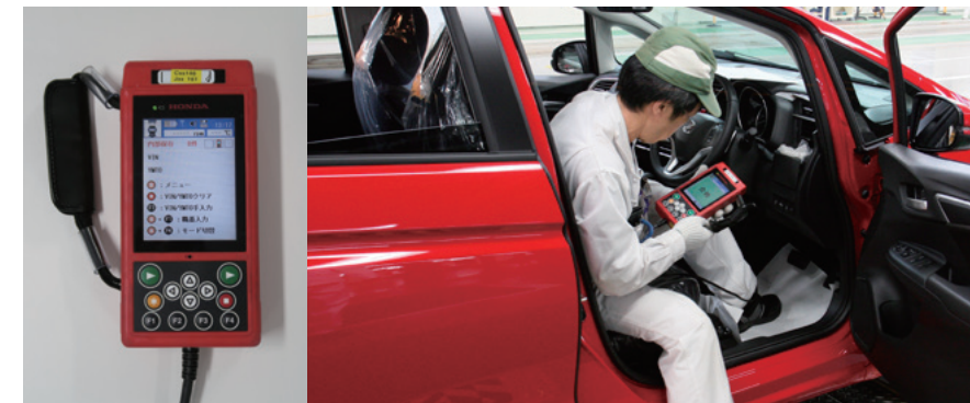
Inspection using LET system
