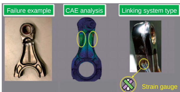
Fig. 12 Failure example, CAE result, linking system type
