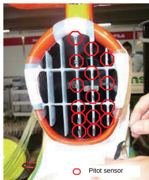
Fig. 4 Pitot sensor position
