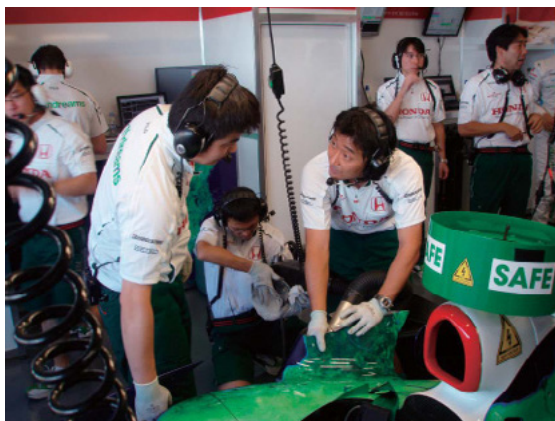
Fig. 5 Checking KERS system
