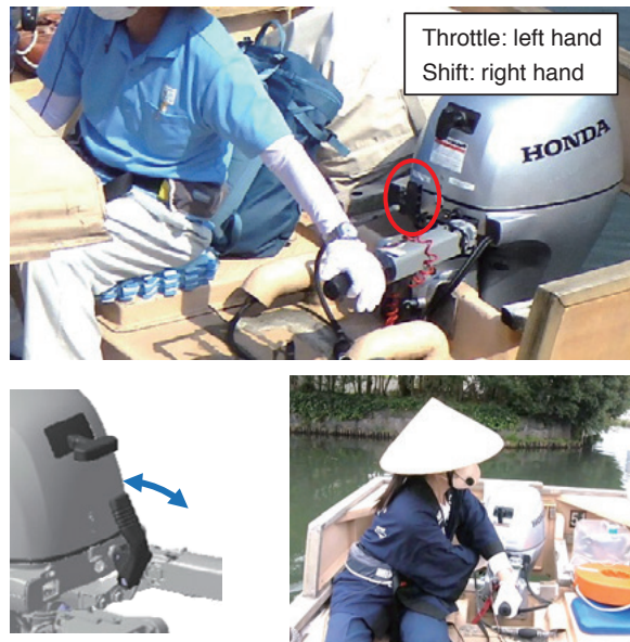
Fig. 10 Conventional method of shift switching
