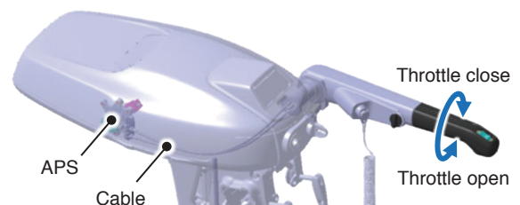
Fig. 13 APS position in electric outboard motor
