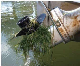
Fig. 17 Tangled algae around propeller
