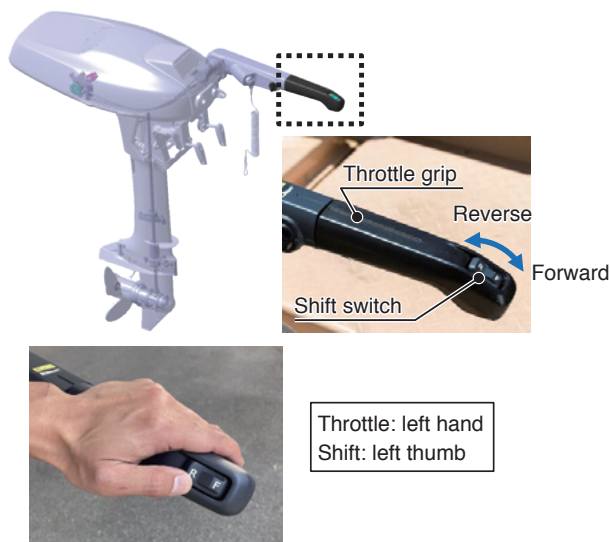
Fig. 11 New method of shifting by alternating switch
