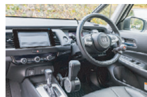
Fig. 1 Adapted vehicle with hand control device
