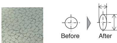
Fig. 5 Measurement method of stamping strain (scribed circle)
