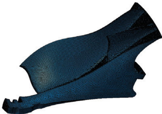
Fig. 4 Structural analysis mesh
