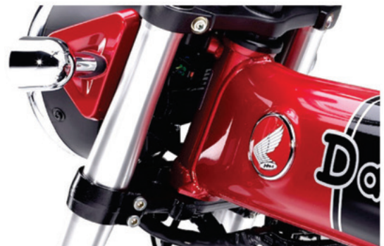
Fig. 21 Simple yet beautiful steering head pipe area without gusset
