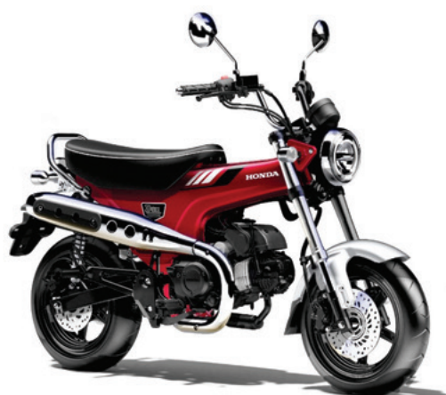
Fig. 13 Pressed steel frame having an optimum volume
