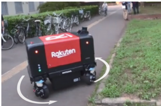
Fig. 19 Turning on spot on narrow road (Minimum turning radius: approximately 700 mm)
