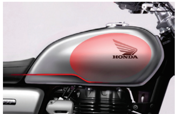
Fig. 14 Character line of fuel tank
