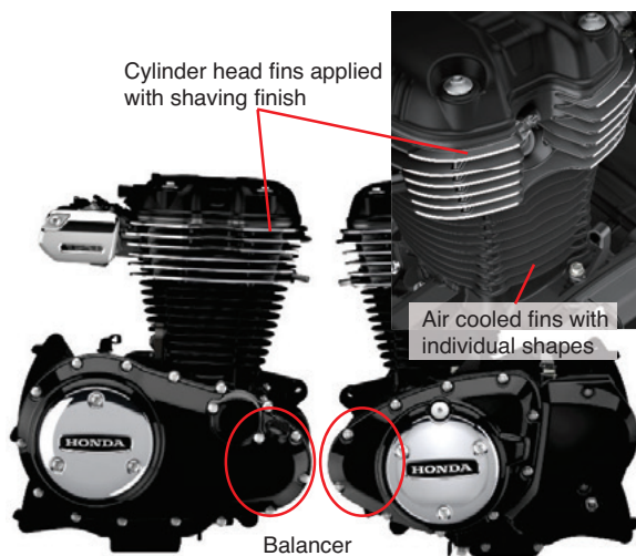
Fig. 19 External design of engine unit
