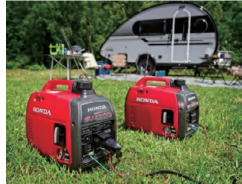
Fig. 17 Example of typical placement location of single-handle portable generator
