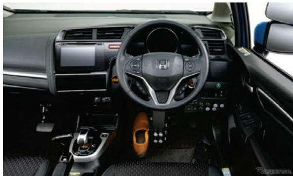
Fig. 7 Honda Franz System for 2017 model year FIT
