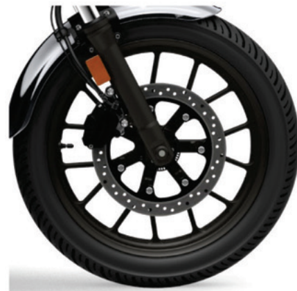
Fig. 21 Exterior design of 14-spoke die-cast aluminum wheel
