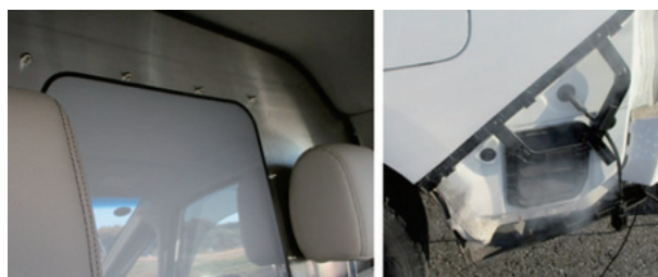
Fig. 8 Smoke leak test
