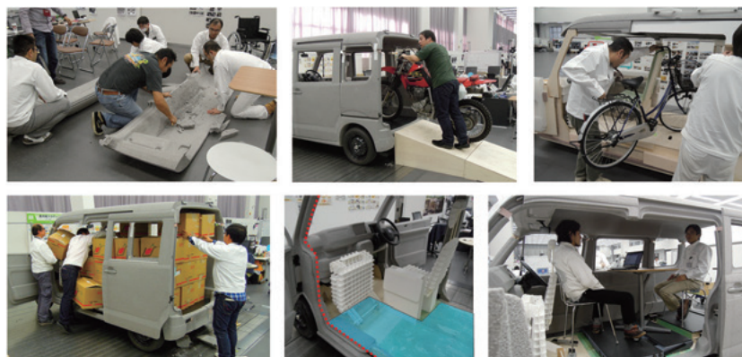
Fig. 5 Package models used in 3D Y-gaya discussions to find ways of “using space completely”
