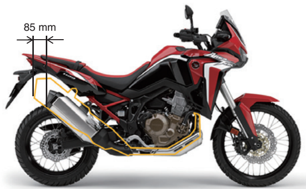
Fig. 11 Comparison of muffler size
