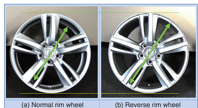
Fig. 1 Appearance of normal rim wheel and reverse rim wheel
