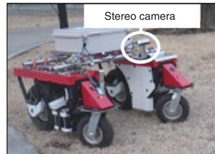
Fig. 6 Test robot with stereo camera
