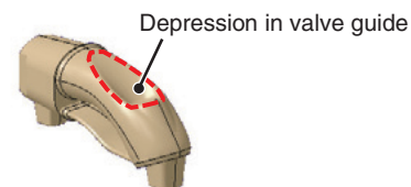
Fig. 28 Place of depression in valve guide
