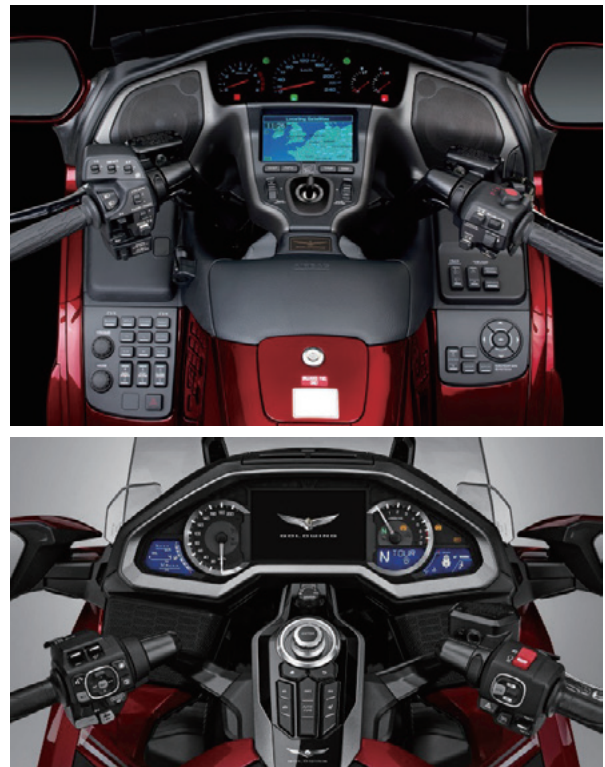
Fig. 5 Arrangement of indicators and control switches (upper side: previous model, lower side: developed model)
