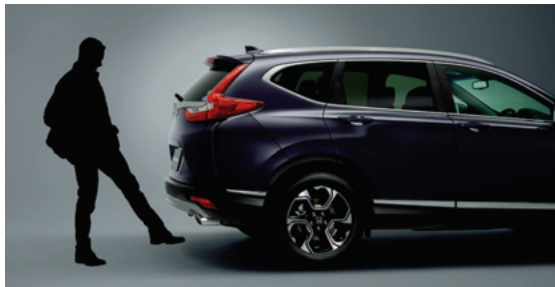
Fig. 3 Power Tail Gate for hands-free access
