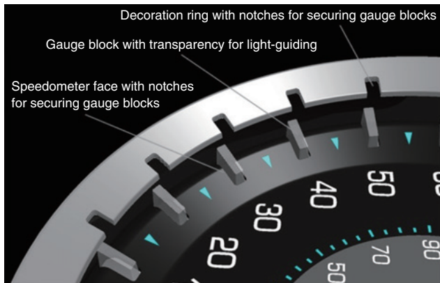
Fig. 21 Exploded view showing gauge ring construction
