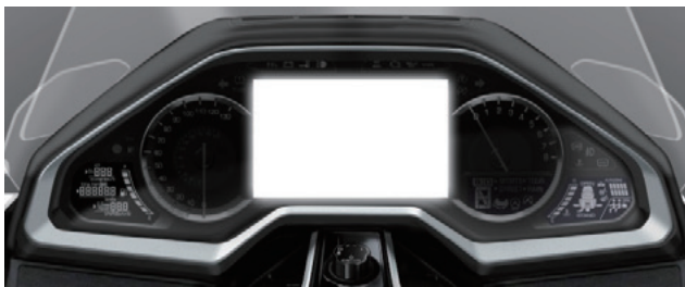
Fig. 13 Residual visual effect caused by excessively high contrast on display screen
