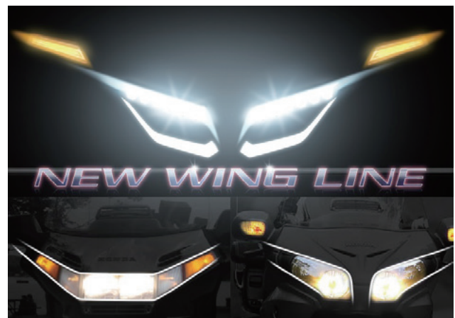
Fig. 3 Wing Line implemented in lighting system design (top: developed design, bottom: previous designs)
