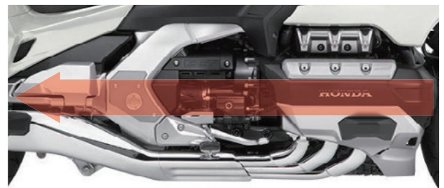
Fig. 16 Integrating components with base character line of the vehicle design
