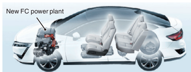
Fig. 1 Schematic drawing of FC power plant for new CLARITY FUEL CELL
