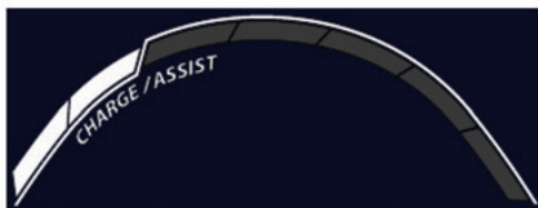
Fig. 23 Charge level indicator (at maximum level)
