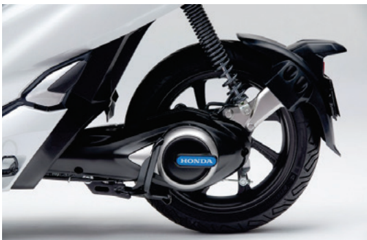
Fig. 31 External view of power unit
