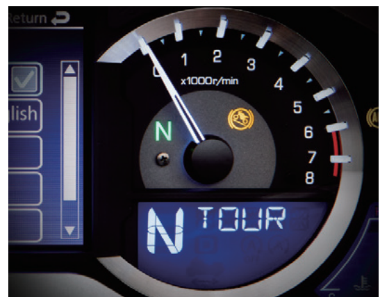
Fig. 20 Analog type tachometer
