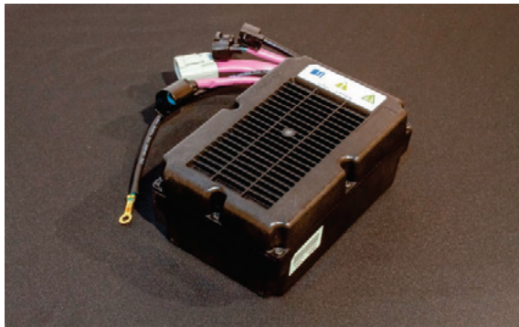
Fig. 14 Appearance of lithium-ion battery pack
