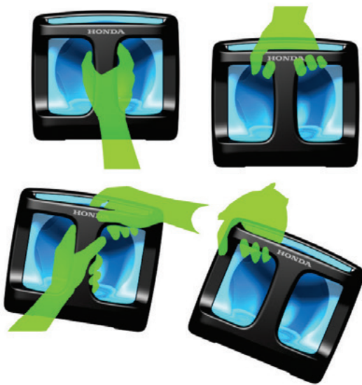
Fig. 17 Methods of hand-carrying battery
