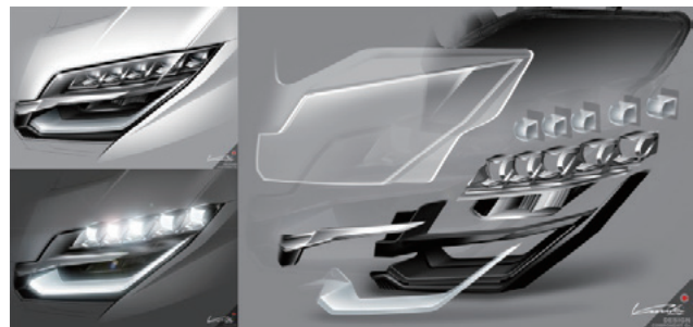
Fig. 10 Drawing showing emitted lights and sketch showing individual components
