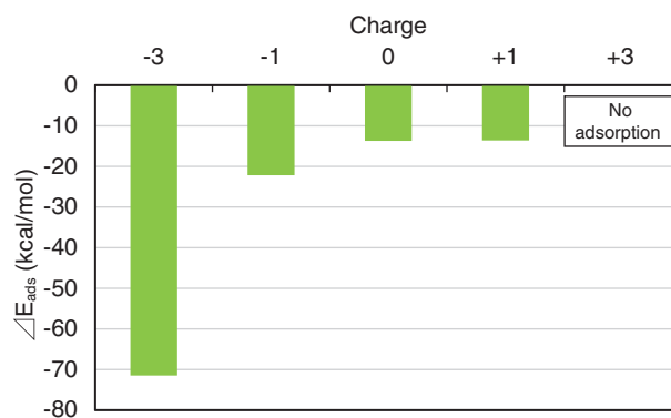
Fig. 10 Oxygen adsorption energy on Pt surface
