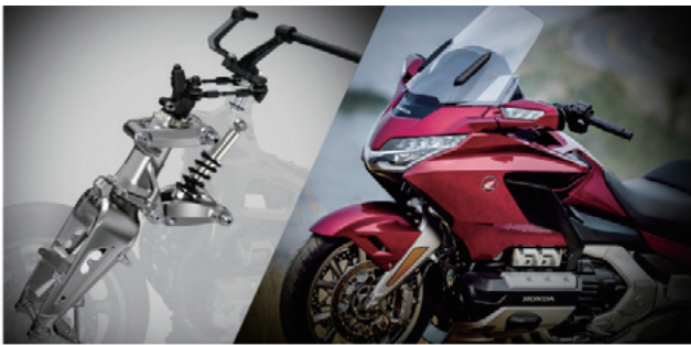
Fig. 16 Double wishbone type front suspension
