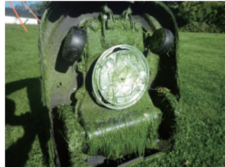
Fig. 10 Grass trimmings on mower underside
