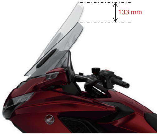
Fig. 26 External view of electronically controlled wind screen
