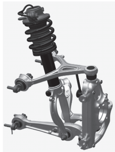
Fig. 2 Double wishbone type suspension for automobiles
