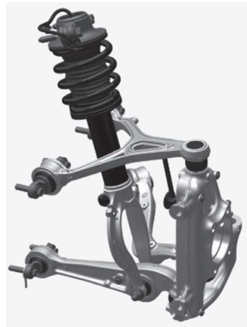
Fig. 2 Double wishbone type suspension for automobiles
