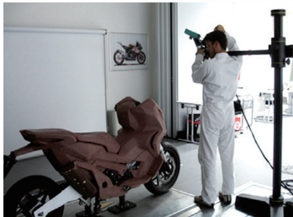
Fig. 10 Riding position checks using clay model before its final finish to investigate dimensions of each part
