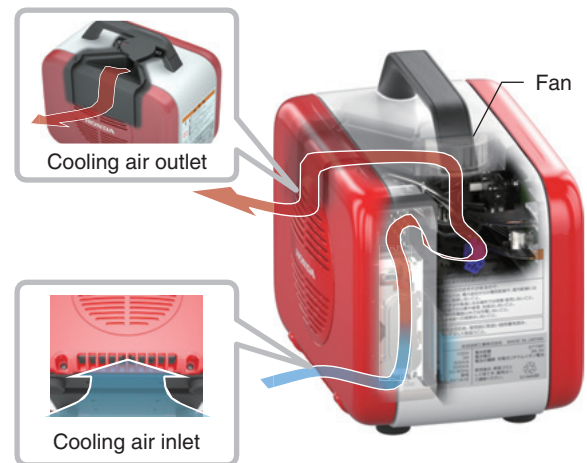
Fig. 14 Cooling air flow
