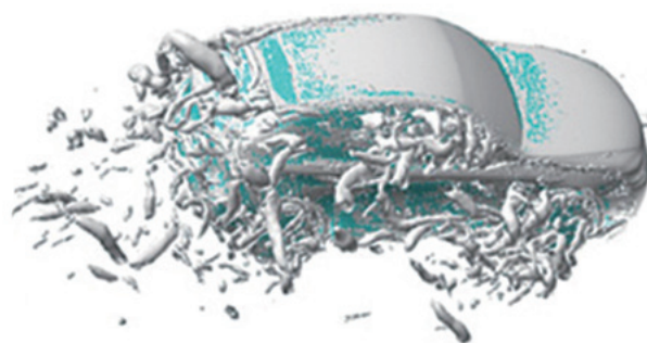
Fig. 4 Crosswind simulation image
