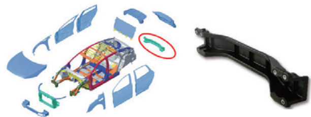
Fig. 9 Thermoplastic GFRP rear bumper beam and location in CLARITY FUEL CELL
