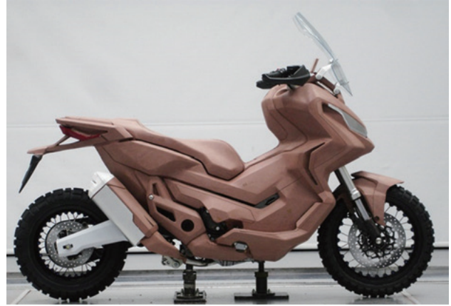
Fig. 11 Completed clay model
