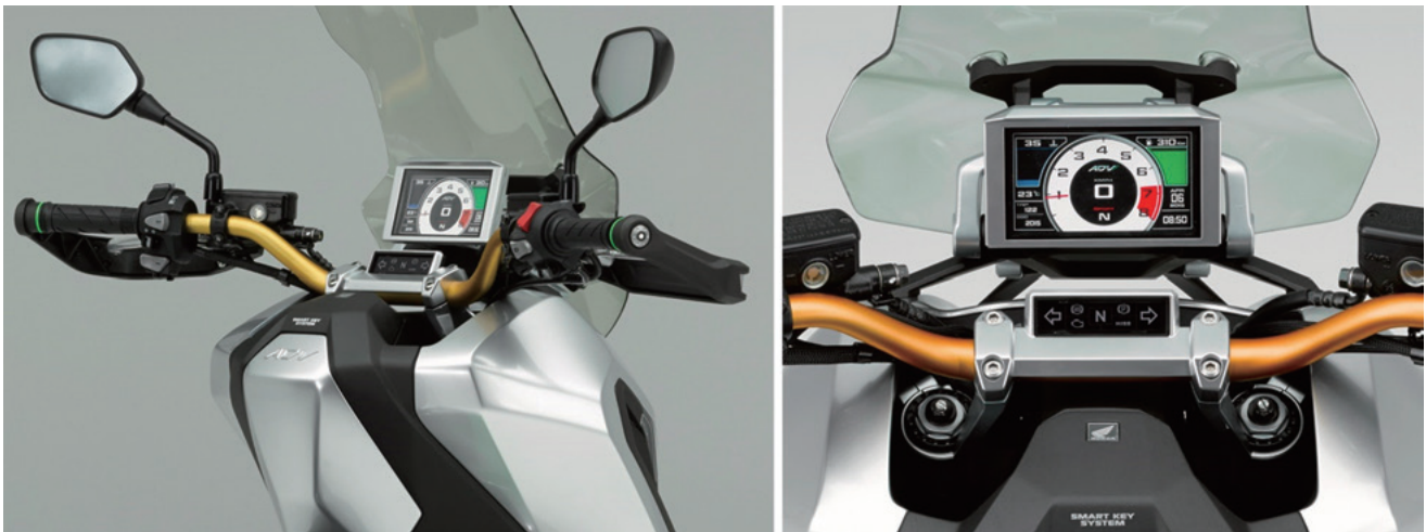
Fig. 14 Display and adjacent area with visibly arranged mechanical parts convenient for commuting
