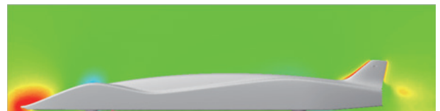
Fig. 12 Shape and section pressure distribution of race car model
