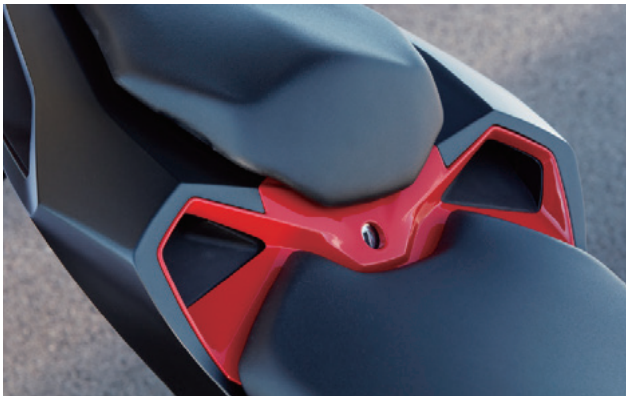
Fig. 32 Air guiding intake openings on rear cowl
