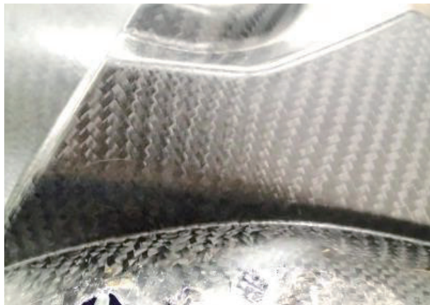
Fig. 10 Appearance of vertical wall side surface when processed with developed method
