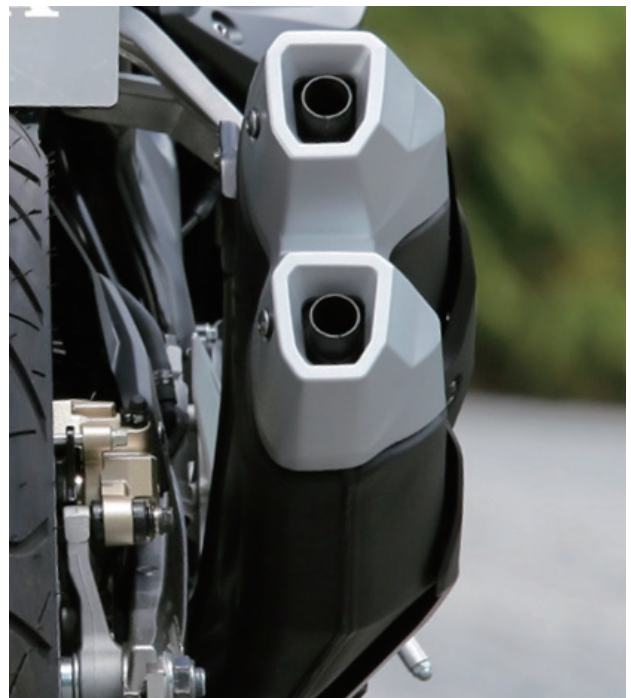
Fig. 35 Twin mufflers with variant cross sections
