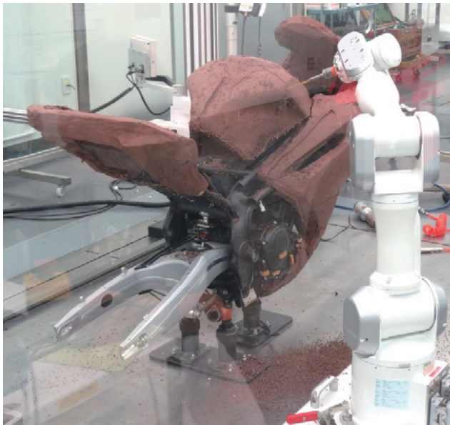
Fig. 22 Production of full scale clay model by numerically controlled clay trimmer
