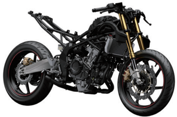
Fig. 9 Computer graphic of body structure skeleton
