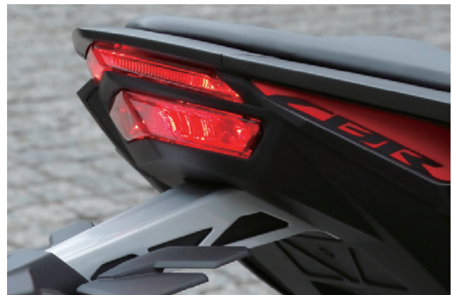
Fig. 31 Two tiered arrangement of upper and lower LED taillights
