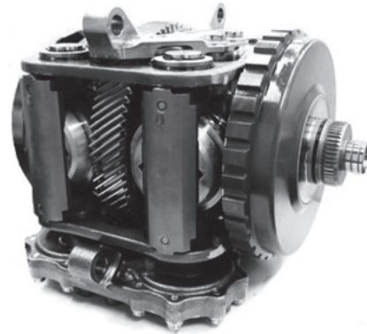
Fig. 3 Double-cavity half-toroidal variator
