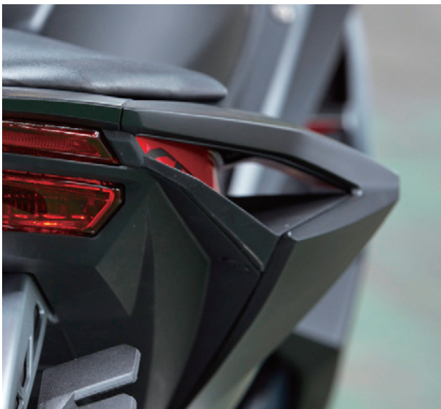
Fig. 33 Air outlets on rear cowl
