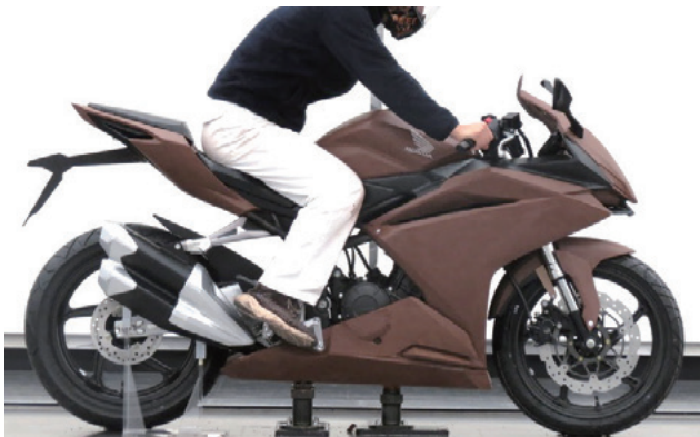
Fig. 23 Lack of sense of unity between rider and vehicle caused by loose distances to components around rider
