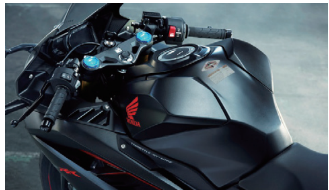
Fig. 25 Shape formation of back portion of tank expressing powerfulness (4-piece tank coverings configuration)
