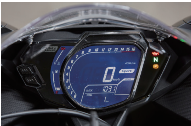
Fig. 36 Large-sized fully digitized gauge unit
