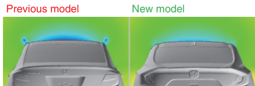
(b) Pressure difference between C-pillar and roof
