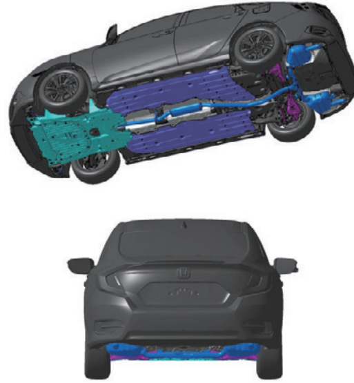
Fig. 8 Aerodynamic treatment on new CIVIC underfloor
