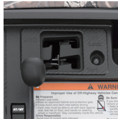
Fig. 17 Drive mode select lever
