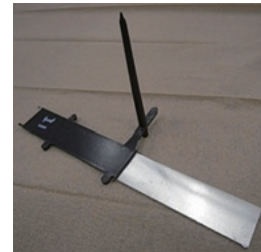
Fig. 9 Specimen of joined CFRTP and Al alloy
