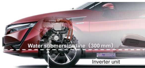
Fig. 21 Inverter mounting position
