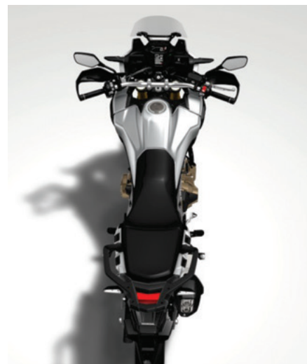
Fig. 13 Streamlined seat shape that helps smooth actions of a rider
