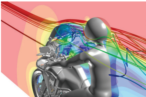
Fig. 15 Air streams around the fairing and the rider
