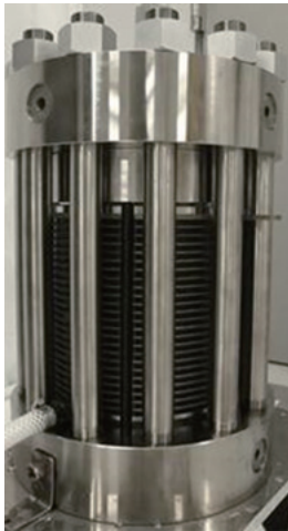
Fig. 12 Photograph of 70 MPa differential-pressure water electrolysis stack
