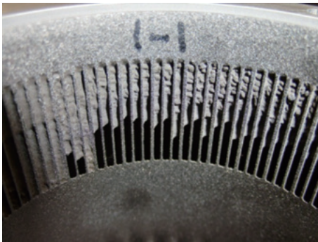
Fig. 15 Congealed powder remaining after machining work to remove reinforcing ring
