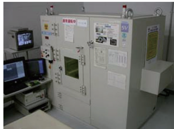
Fig. 23 Shimadzu Micro-focus X-ray CT System (SMX-225CT-SV3)
