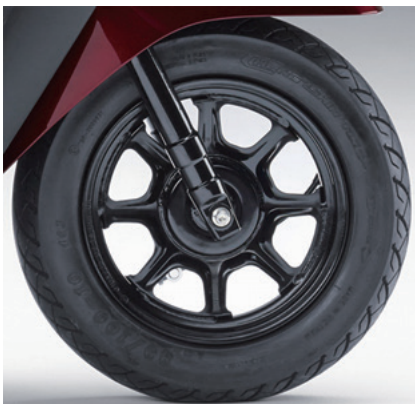
Fig. 18 Steel wheel with spoke like radial pattern
