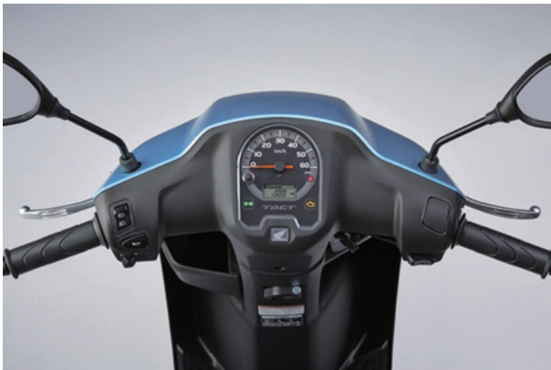
Fig. 17 Simplified speedometer design for good visibility
