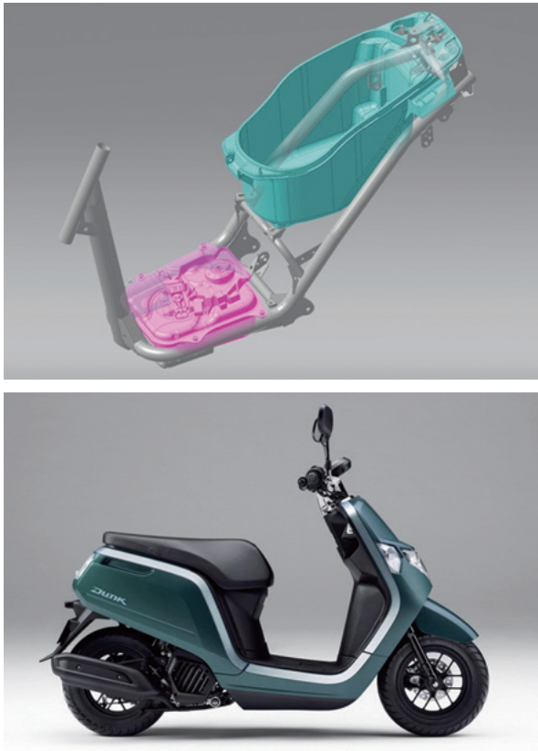
Fig. 7 Body frame configuration and exterior view of the Dunk
