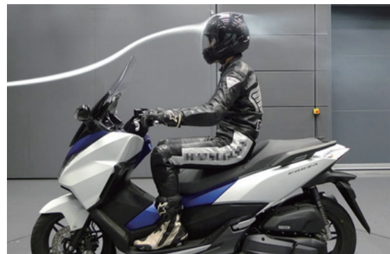
Fig. 15 Design verification using wind tunnel
