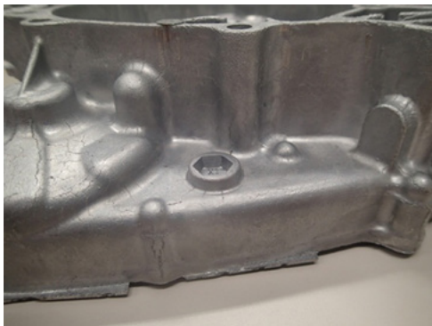
Fig. 26 Raw material appearance after 10000 shots
