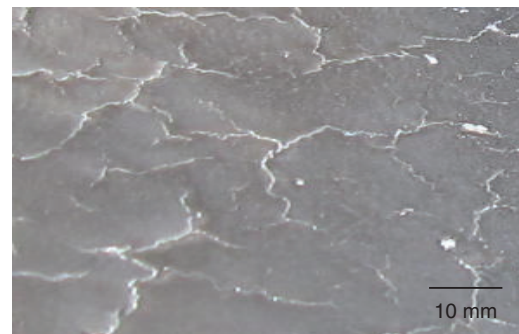
Fig. 17 Heat checks occurred on die surface
