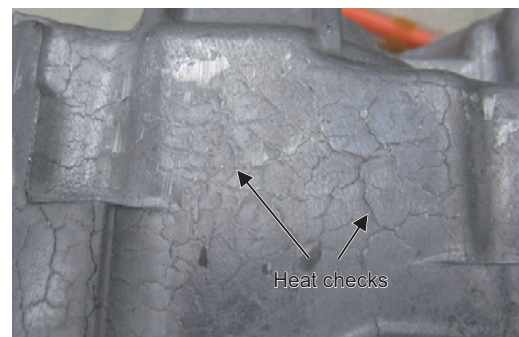
Fig. 16 Transferred heat checks
