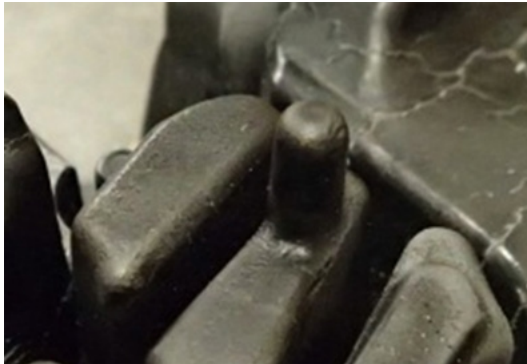
Fig. 25 Shape section after 10000 shots
