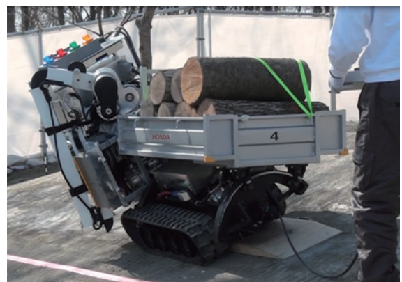
Fig. 16 Traveling on slope using overturn suppression
