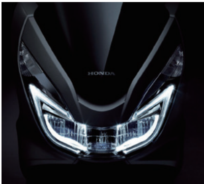
Fig. 6 Application of light guiding panel in the PCX, 2014 year model
