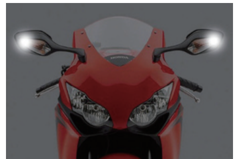
Fig. 4 Front position lights (at rear view mirror) in the CBR1000RR, 2008 year model
