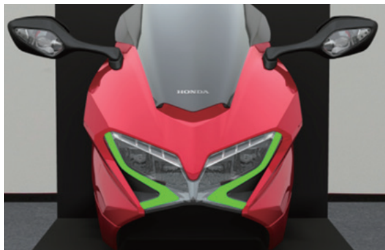
Fig. 10 Applied light guiding panel (shown in green color)
