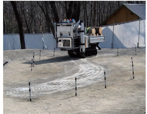
Fig. 9 Automatic traveling by electromagnetic navigation
