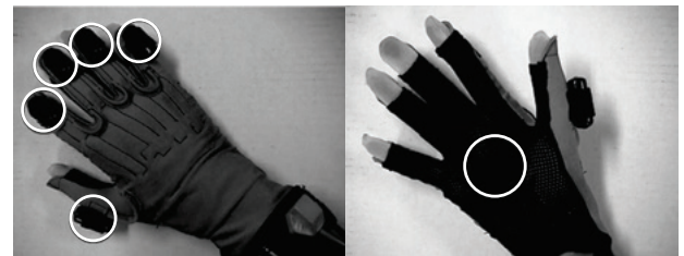
Fig. 1 Vibrators on right-hand glove. Five small motors are placed at circled locations on the tops of the fingers and one on the palm.
