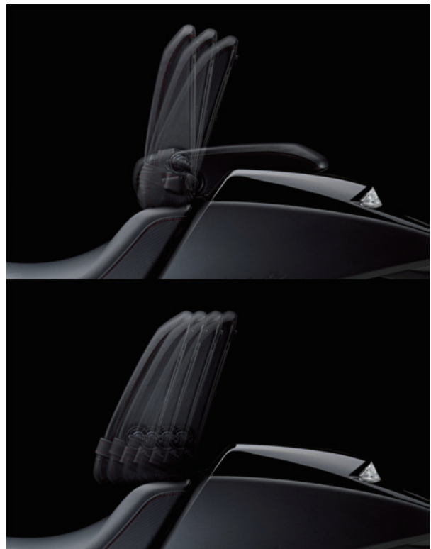
Fig. 10 Upright positionable pillion (4 angular positions including 3 upright positions with longitudinal adjuster)
