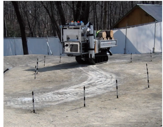
Fig. 9 Automatic traveling by electromagnetic navigation
