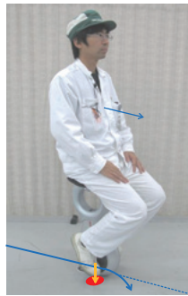
Fig. 9 U3-X turning procedure using toe
