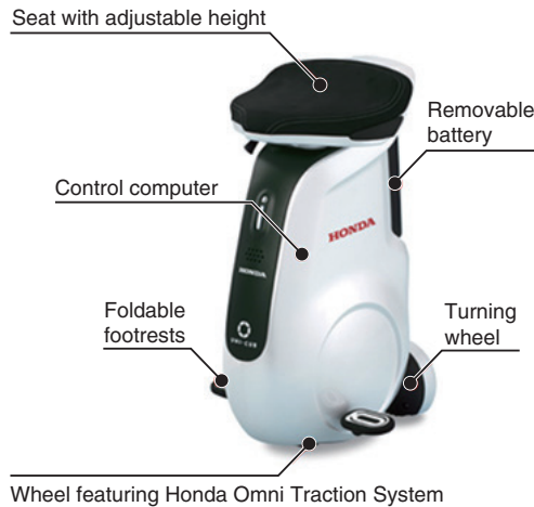
Fig. 5 External view of UNI-CUB
