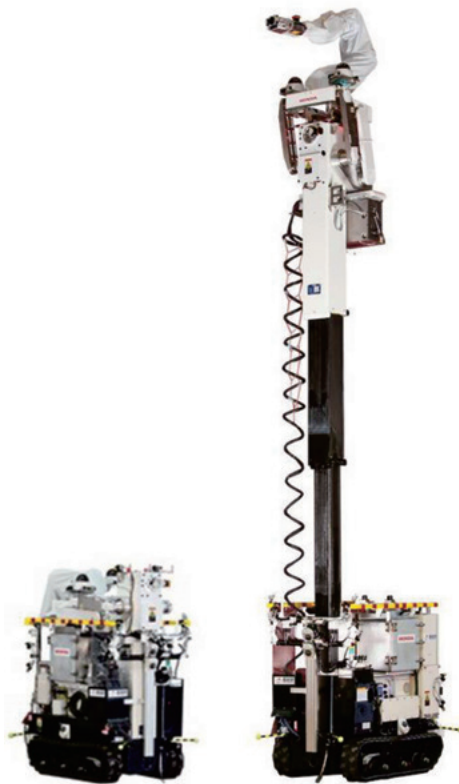
Fig. 1 High-Access Survey Robot The driving posture (left) and higher posture (right)
