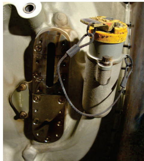
Fig. 2 Fire exposure area of oil tank after test
