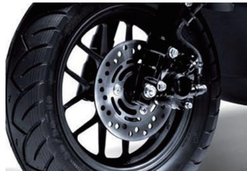
Fig. 19 Front disc brake with CBS and aluminum die-cast wheel
