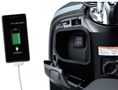
Fig. 17 Charging socket for smartphones equipped in glove box
