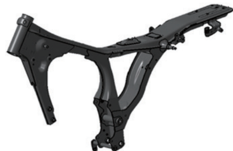
Fig. 2 Mono-bone frame of 2013 model year CG150
