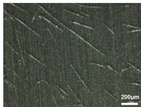
Fig. 5 Glass fillers appeared on surface of PA
