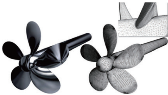
Fig. 4 Propeller CAD model (left) and computational mesh (right)
