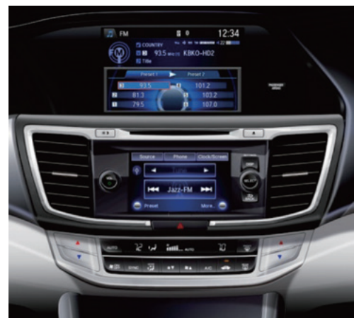
Fig. 23 Audio with touch screen and 8-inch display
