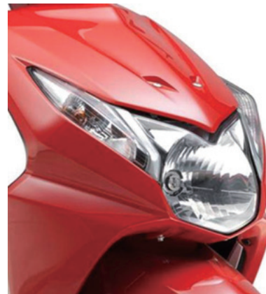
Fig. 6 Integrated headlight unit with turn signals
