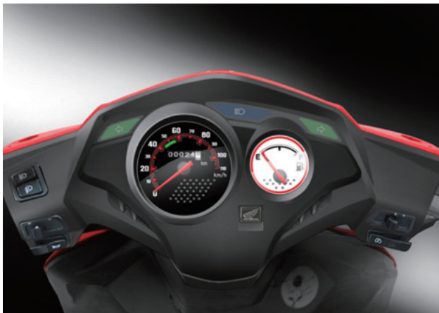
Fig. 8 Concept sketch of asymmetrical meter panel design
