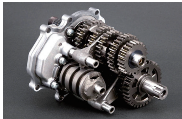
Fig. 11 Cassette type transmission
