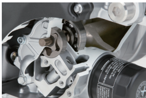
Fig. 12 Oil pump driven via balancer shaft
