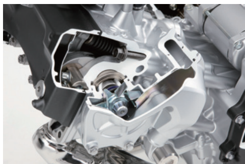
Fig. 13 Water pump driven via camshaft
